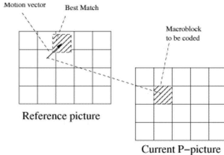
The motion vector has a pixelic precision for luma component and half pixel precision for chroma component due to chroma subsampling. Therefore Chroma needs to be interpolated to access sub pixels (refer to h.264 specification).
