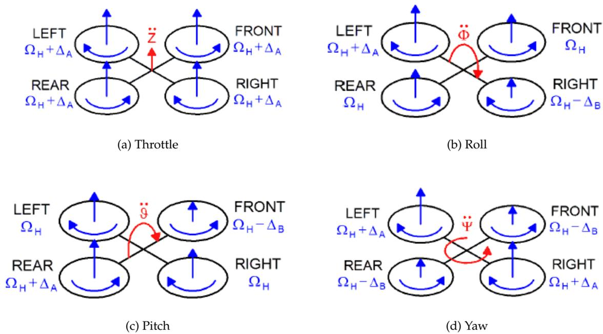
Figure 2.1: Drone movements
