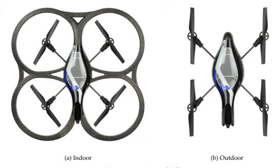
Figure 2.2: Drone hulls
