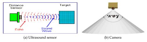
Figure 2.3: Drone Sensors
