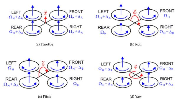
Figure 2.1: Drone movements
